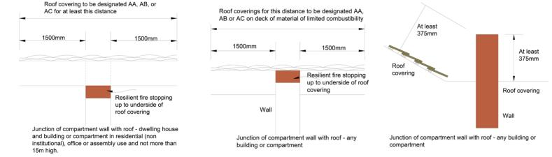
Figure 13: Typical fire stopping details
