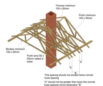
Figure 8: Roof trusses trimming around a chimney
