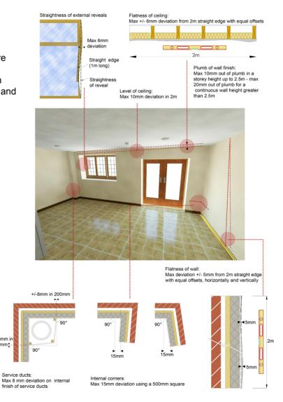
Figure 6: Maximum deviation in walls and ceilings
