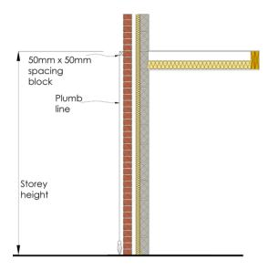
Figure 4: Plumb of wall: storey height
