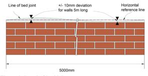
Figure 2: Level of bed joints
