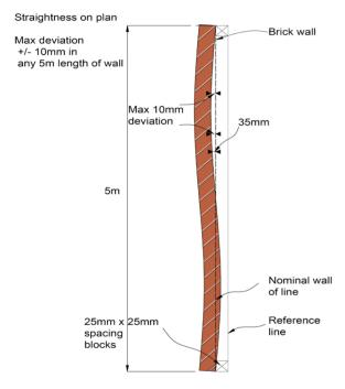
Figure 1: Brickwork: straightness on plan
