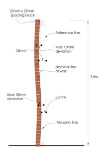
Figure 5: Straightness in section
