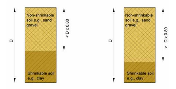
Figure 12 and 13: Foundation depth required to be taken down using foundation calculator and plasticity index of underlying clay
