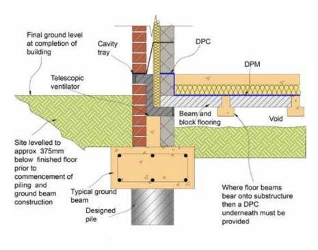
Figure 19: Pile and beam detail
