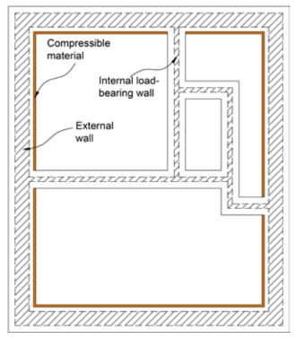
Figure 9: Plan of heave protection to a mass filled foundation
