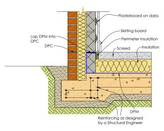
Figure 20: Typical raft foundation design
