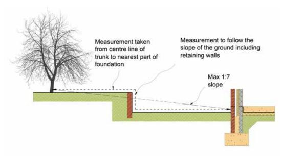
Figure 11: Measuring foundation distance on sloping sites
