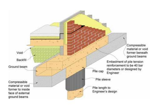
Figure 10: Heave protection: Section of pile and beam foundation
