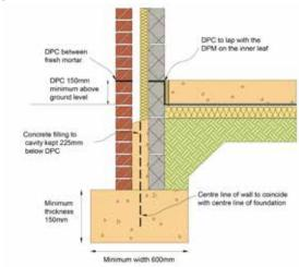
Figure 14: Typical strip foundation
