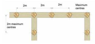
Figure 4: The intersection of adjacent reinforced concrete strips
