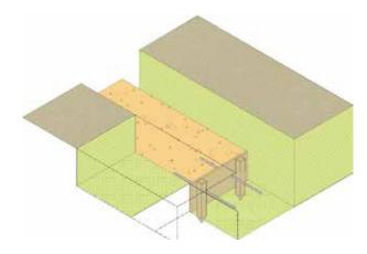
Figure 16: Using reinforcement bars across a joint
