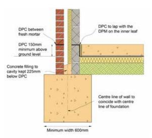
Figure 15: Typical mass fill foundation
