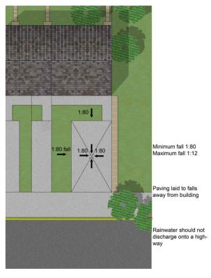
Figure 2: Drive and pathway drainage
